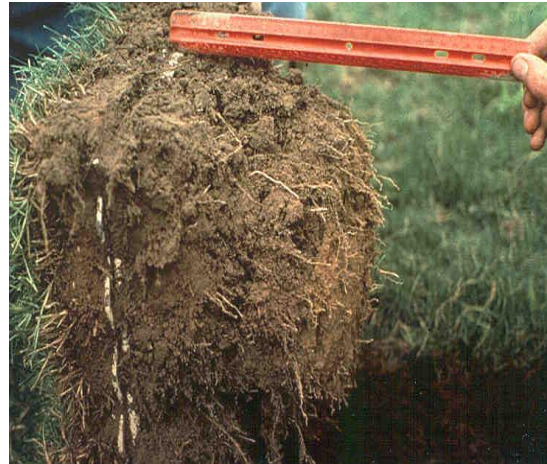
Root frame used to evaluate rooting by measuring force required to pull the frame
